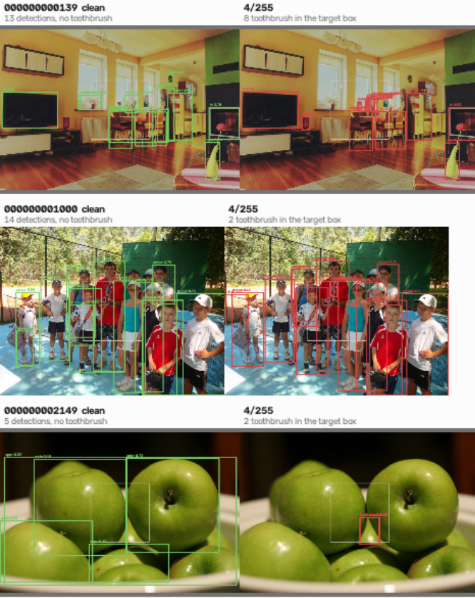
Fig. 17. Targeted object insertion on three scenes; the chosen class is toothbrush and the budget is printed on each panel. Left: the unmodified photograph. Right: the same photograph after a bounded attack that raises the chosen class inside the chosen target box, with the inserted detection drawn. The perturbation is confined to the stated L-infinity budget and is not visible at this scale; the inserted box carries a confidence above the reporting threshold, so nothing downstream distinguishes it from a real one.
