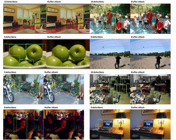
Fig. 7. Eight scenes at a fixed budget of 1/255, clean above and attacked below. The effect is not particular to a scene type: indoor and outdoor, crowded and sparse, large objects and small all lose their output at the same budget, which is what makes the rate in Table 5 a property of the model rather than of the images we happened to select.
