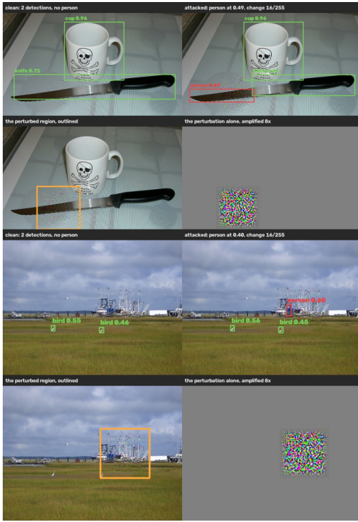
Fig. 30. Image-specific perturbation on two held-out photographs containing no person. For each photograph the upper row gives the original and the attacked file, with the inserted person in red and the largest pixel change stated; the lower row outlines the perturbed region, because it is otherwise not locatable, and shows the perturbation alone amplified eight times. The perturbation adds to the photograph’s own pixels: the changed region keeps a structural similarity of 0.85 to the original and the whole file 0.98 (PSNR 38 dB), while the detector’s output changes.
