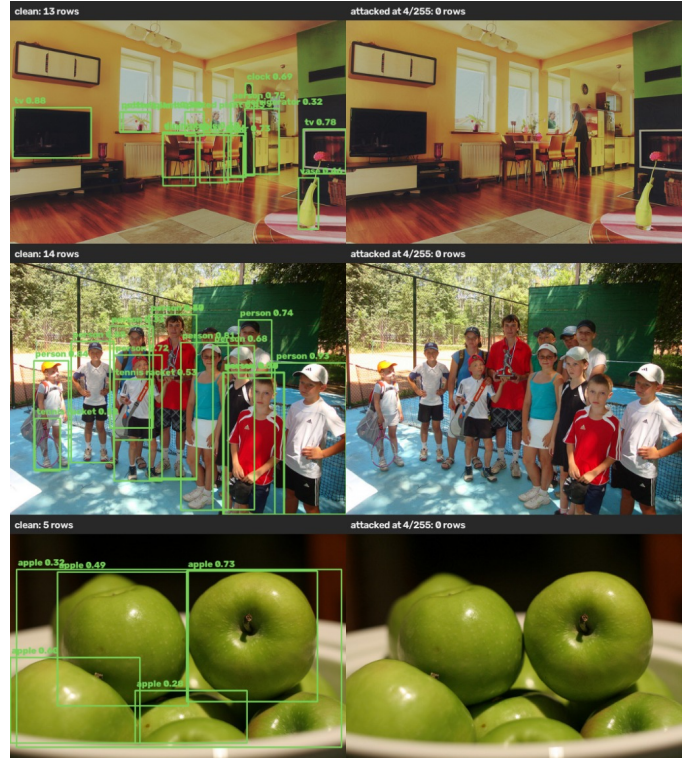
Fig. 23. Duplicate injection. Left: the clean image, one detection for the object. Right: the attacked image, two overlapping detections of the same class above threshold for the same object. Both carry confidences above the reporting threshold, so a consumer that counts objects from the raw output reports one too many with nothing to indicate a fault.
