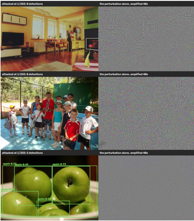
Fig. 8. The perturbation at 1/255 beside the photograph it is added to, amplified so that it can be seen at all. At true scale it is one part in 255 of the pixel range. The amplified panel shows spatial structure; the noise baseline of Section V-B, at thirty times this budget, has none by construction.
