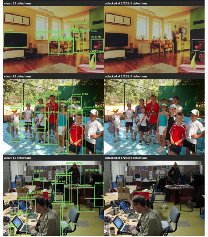
Fig. 6. Object vanishing on three scenes from the tuning split. Left: the unmodified file with everything the detector reports. Right: the same photograph after a bounded gradient attack at 1/255, scored through the same pipeline, reporting nothing. The perturbation is one grey level per pixel and is not visible at this scale, which is the availability result in visual form: the failure is not preceded by degraded boxes or falling confidences.
